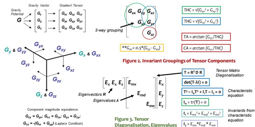
Figure 1. Gravity and Gradient Components
